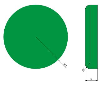
Figure 1: 3D printed mock wearable device
